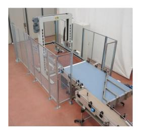
Semiautomatic machine for bottle and jar depalletising, featuring low-level discharge and pallet on the floor
