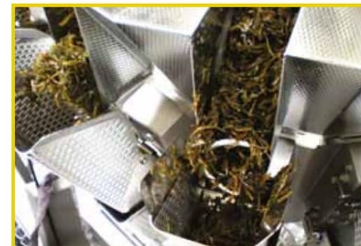
Cabinplant screw feeding multihead weigher is specially designed to handle delicate thread-like products, e.g. shredded marinated vegetables.
