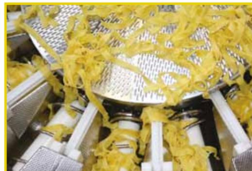
Screw feeding multihead weigher, type 30-14. Core and rollers ensure gentle transfer of fragile product.
