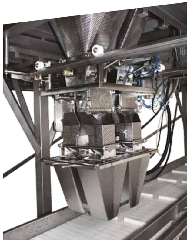
Distribution tool, 2x2, for packing of ready meals in trays of fixed weight.
