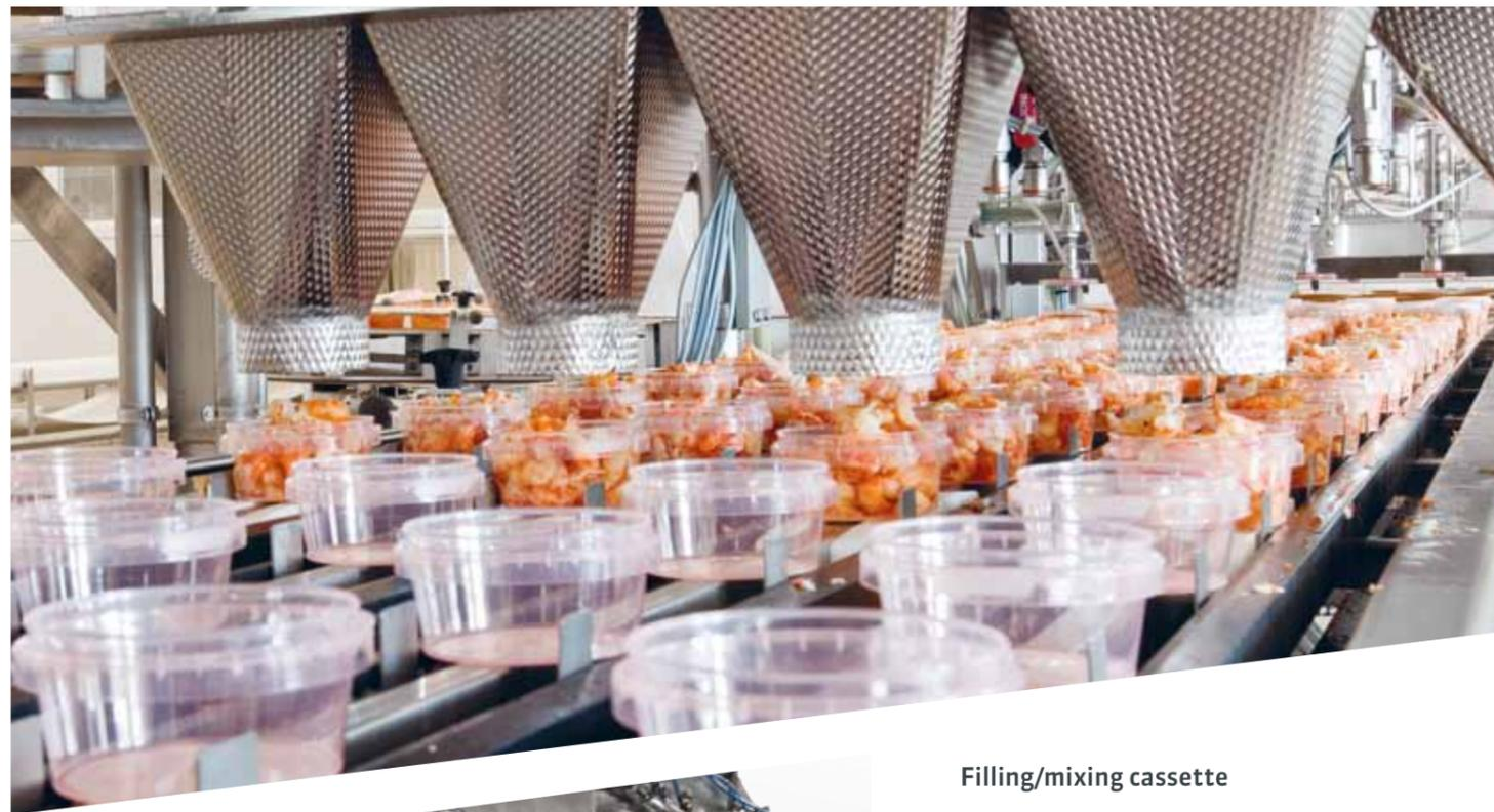
In many cases, the challenge of using multihead weighing is the combination of the multihead weigher with the subsequent packing equipment.
