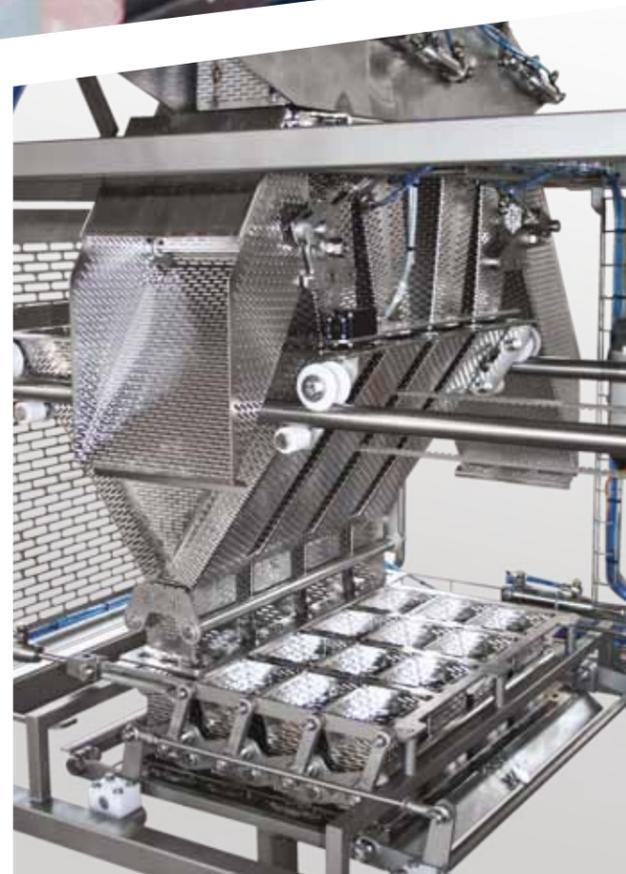
Distribution tool, 4x4, for thermoformed trays.
