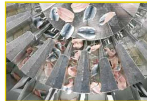
Assembling hopper with anti-sticky surface.
