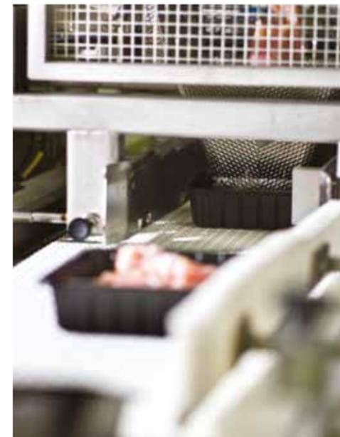
The tool distributes and guides the product from the timing hopper to the final container – safely, quickly and without spillage.
