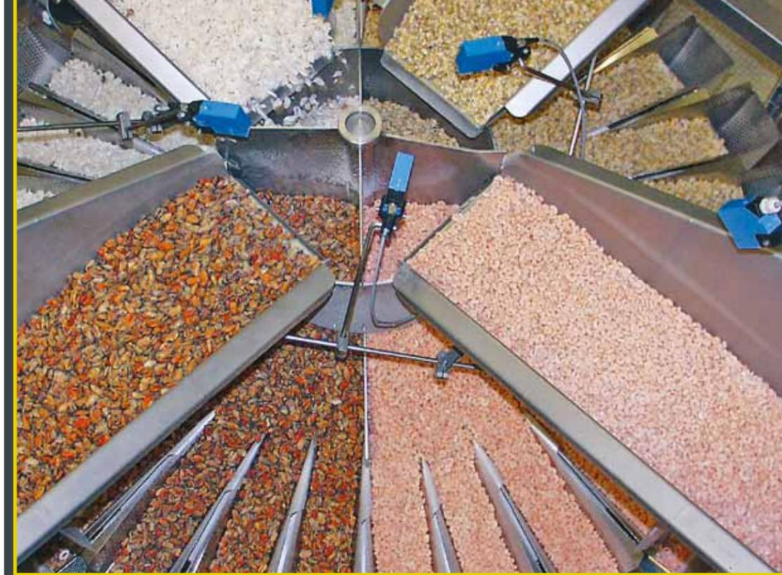
Multihead weighing of accurate mixes of four different seafood products: Two types of mussels, shrimp and squid.
