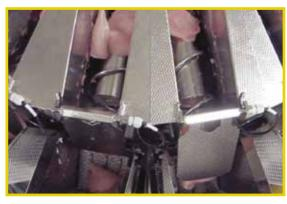
Sensor gates reduce no. of empty weighing pans as well as duplets and triplets in the weighing pans.
