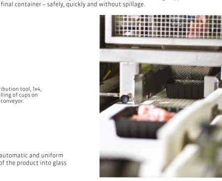
The tool distributes and guides the product from the timing hopper to the final container – safely, quickly and without spillage.
