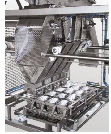
Distribution tool, 4x4, for thermoformed trays.
