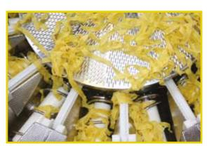
Screw feeding multihead weigher, type 30-14. Core and rollers ensure gentle transfer of fragile product.
