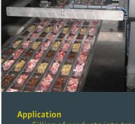
Filling of products into trays formed by a thermoforming machine or into trays on a step conveyor
