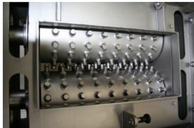
Spikes pulled by a gear motor
