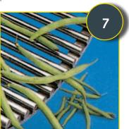
The larger beans going over the end of the grader are cut according to the requirements of the individual processor, either crosswise or lengthwise (French style)
