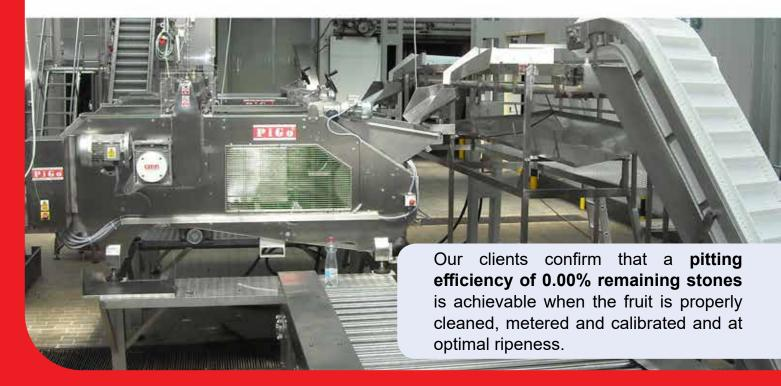
**UP TO 5 TIMES THE CAPACITY OF ANY COMPETITIVE SYSTEM**. A defining characteristic of the PG103 is the fruit distribution system. Though it has extra large plates, the machine's proprietary distribution system ensures that the plates are consistently filled to almost 100%. The pitting plates maintain full capacity even at optimal pitting cycle rates of 60 cycles per minute.
