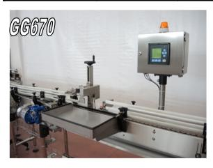
New measuring system with detection effected without contact between sensor and cap. It detects the vacuum presence and/or the lack of cap on the filled jars.
