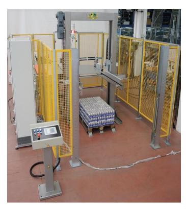
Semi-automatic machine for carton palletising, with low-level loading and pallet at floor level
