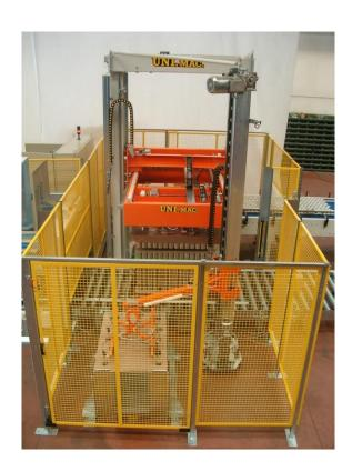
Automatic machines equipped with magnetic head for palletising (or depalletising) empty and full cans, full jars and bottles featuring low-level loading (unloading)
