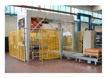
Automatic machines with magnetic head for palletising (or depalletising) empty and full cans, full jars and bottles with metal caps, featuring low-level loading (unloading)
